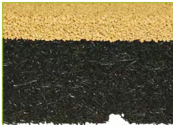
The cross section shows the dual-layer construction with the solid-coloured EPDM layer.
